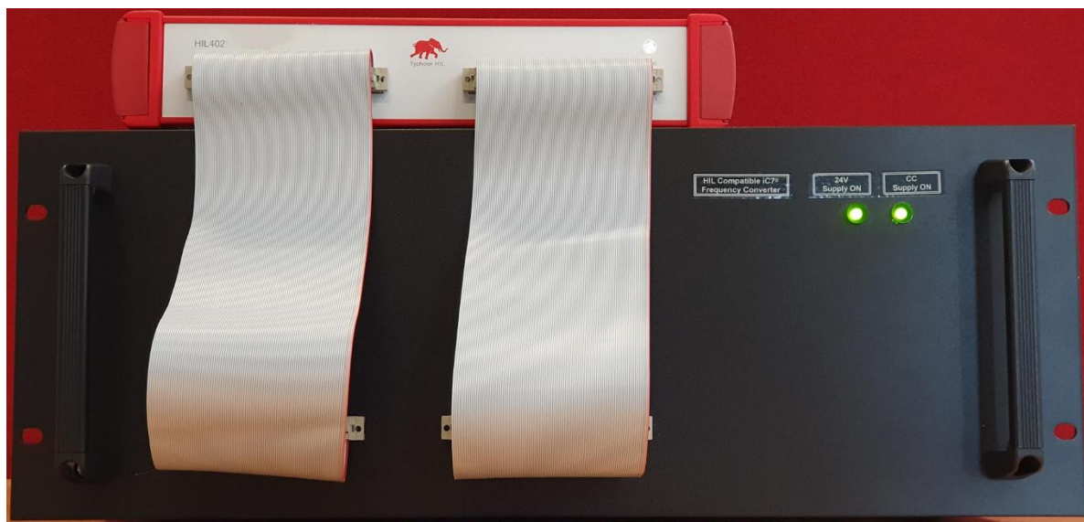
Figure 1: Front with ribbon-cables to HIL404 device.
