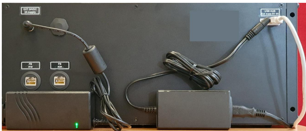
Figure 2: Rear with connection for main power supplies, USB for access to the service-port of iC7 control unit, and Ethernet based Fieldbus for control unit.
